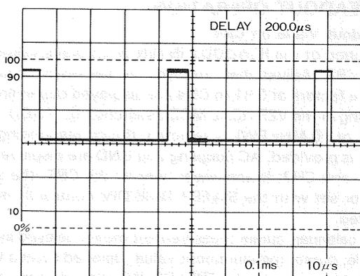
Though the delay time, 200μs, is set at the point of 2 div., the trigger point after it is at the point of 4.3 div.; consequently, the part from 4.3 div. is intensity-modulated (for magnification).
