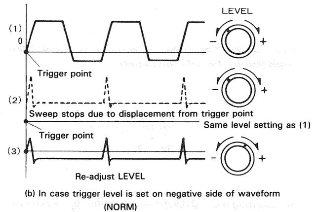
(b) In case trigger level is set on negative side of waveform (NORM)
