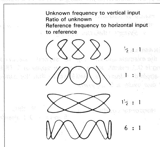
Fig. 51 Lissajous' Pattern used for Frequency Measurement
