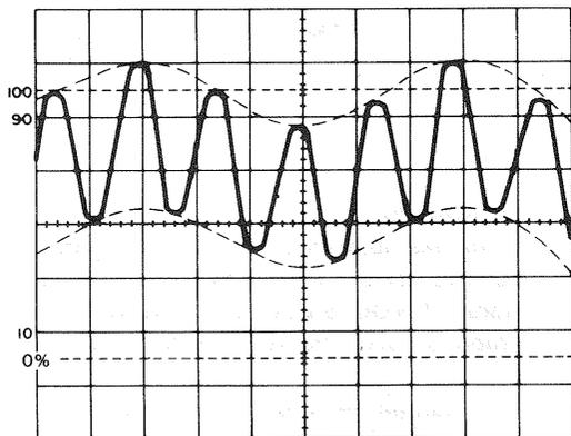
Signal containing undesired component
